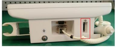
Figure 5-11 Console SD card interface
