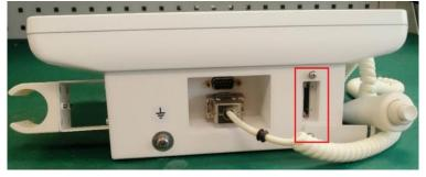
Figure 5-11 Console SD card interface
