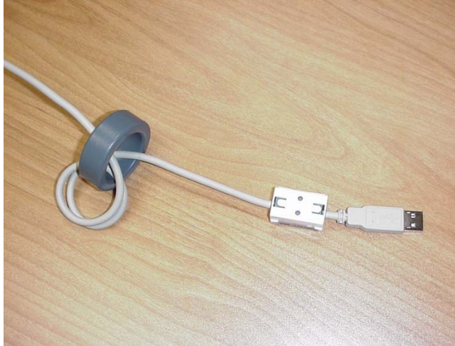
Figure 10- Example of a USB Cable Using Ferrites
