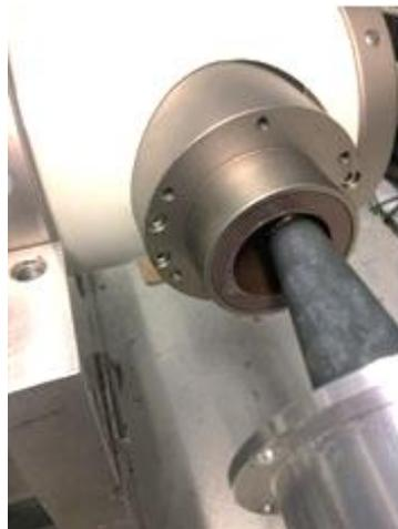
Insert HV cable plug in tube receptacle
