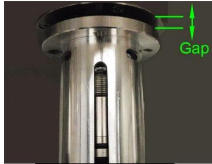
Adjust flange for proper gapping
