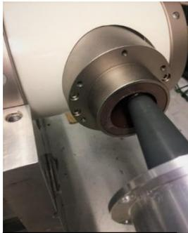
Insert dry HV cable plug into X-ray tube
