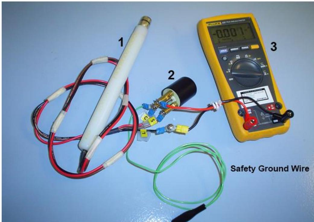
C=Common Connection, L= Large Filament Connection, S= Small Filament Connection
