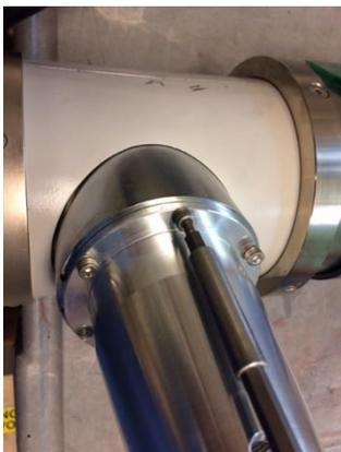
Tighten cable flange screws
