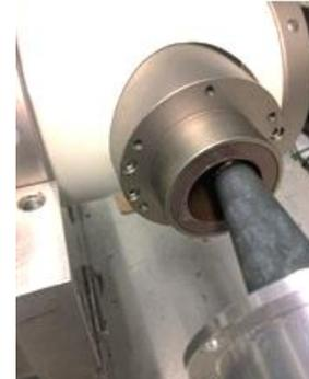
Insert HV cable plug in tube receptacle
