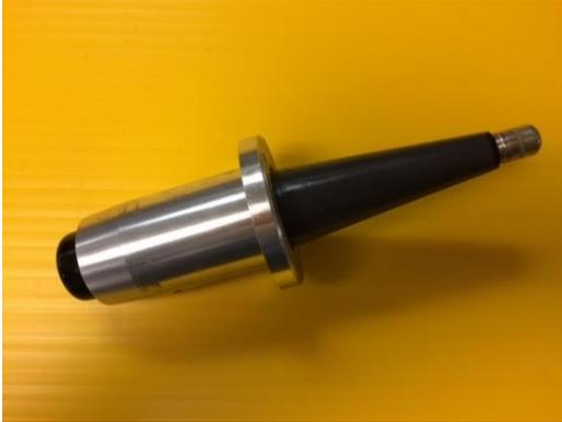
R24 test plug useful for evaluating or troubleshooting XRV160 model generators or X-ray tube functionality. The plug is inserted into the high voltage receptical and allows for operation of the XRV Generator without the X-ray tube load.
