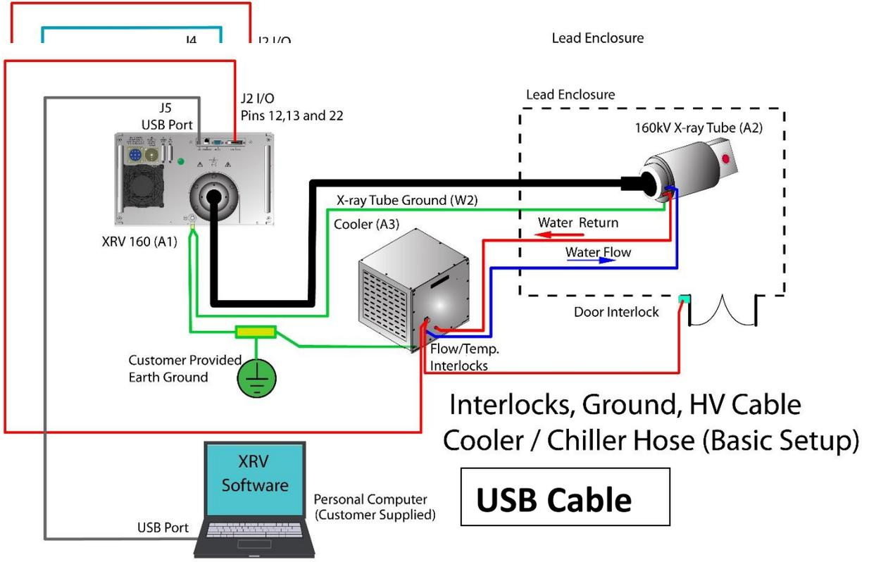
**Interlock, Communication Connections (Unipolar Basic):**
