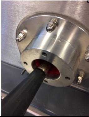
Insert dry HV cable plug in XRV receptacle
