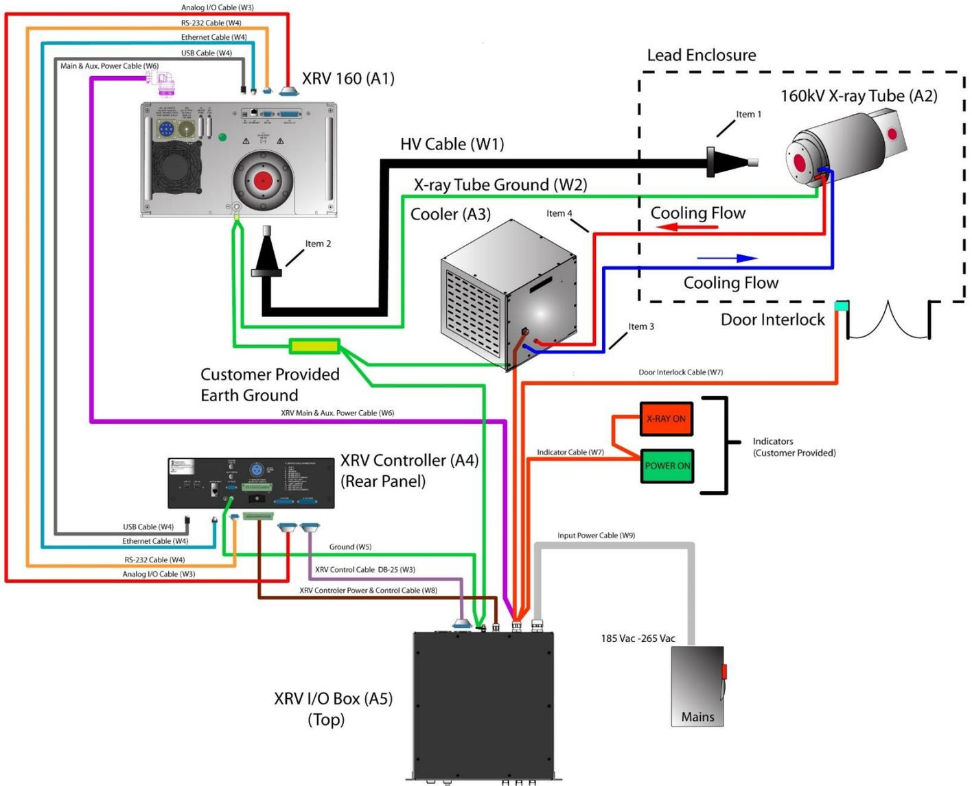
Typical Unipolar System with Additional Controller and I/O Box
