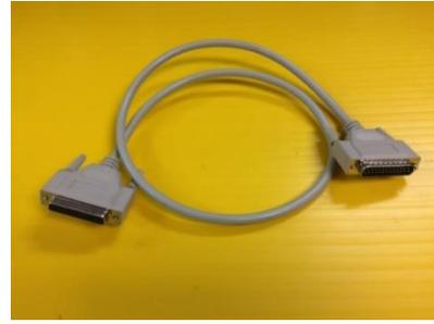
J3 to J7 Anode to Cathode Inverter Control Cable
