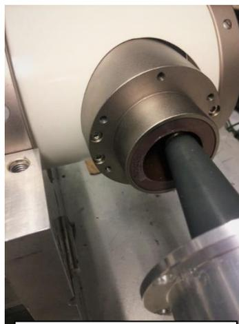
Insert dry HV cable plug into X-ray tube
