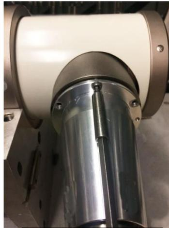
Tighten cable flange screws
