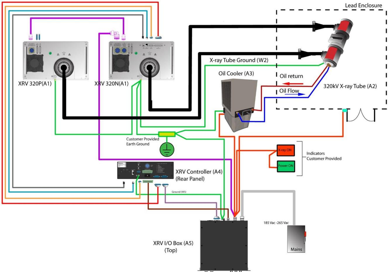
Typical Bipolar System with Additional Controller and I/O Box
