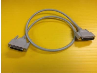
J2 to J6 Anode to Cathode Feedback Cable
