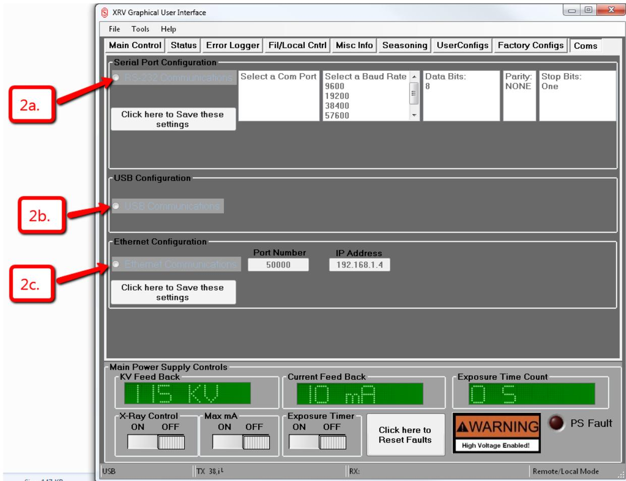
Note: When using the RS232 method of communication, the user must select a Com port, Baud Rate, Data Bits, Parity, and Stop Bits. When using the Ethernet method of communication, the user must select a port number and IP address. Be sure to press the “Click here to save these settings” button when finished.
