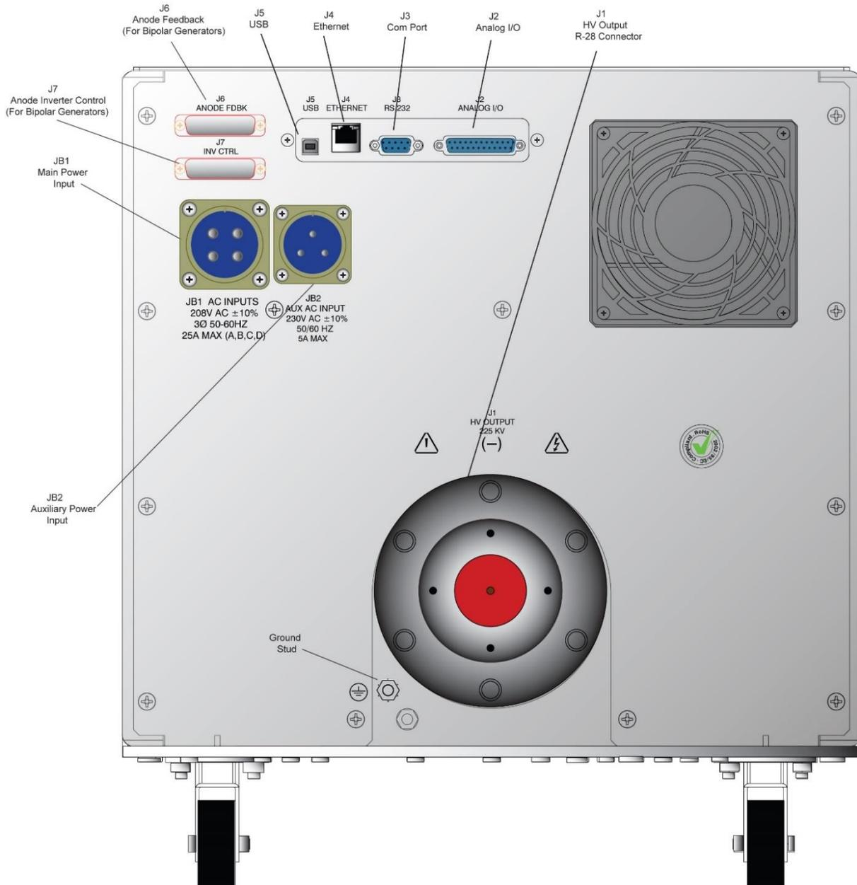
**XR225kV 208Vac 3Ø 6kW Unit**
