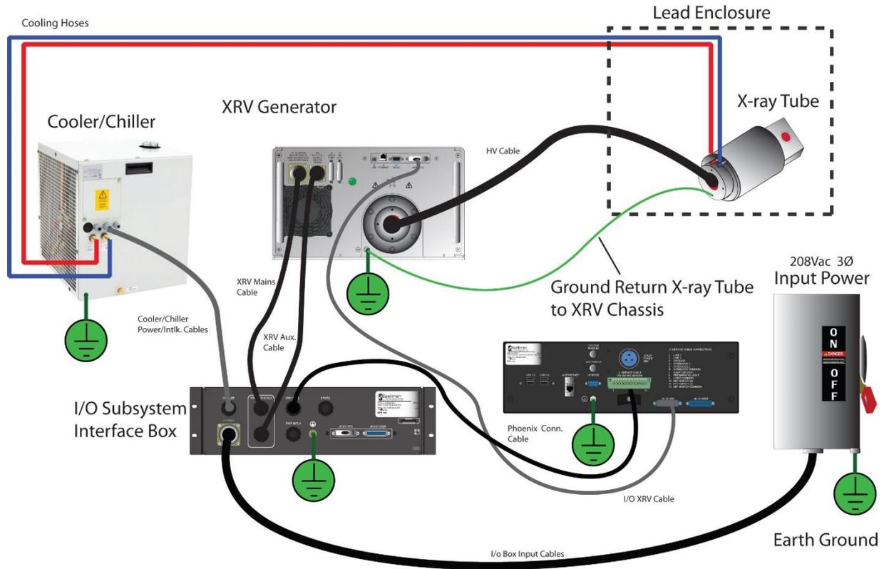
XRVC Controller, I/O System Interface Box, Cooler/Chiller, XRVC Generator and X-Ray Tube Setup for 6kW System
