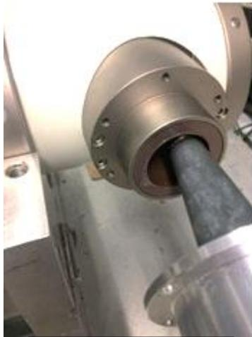
Insert HV cable plug in tube receptacle
