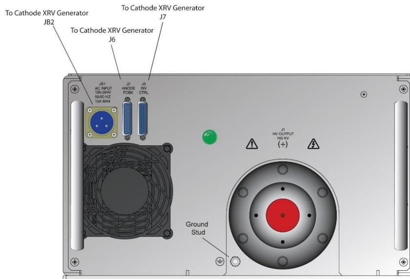
Anode Power & Feedback Connections
