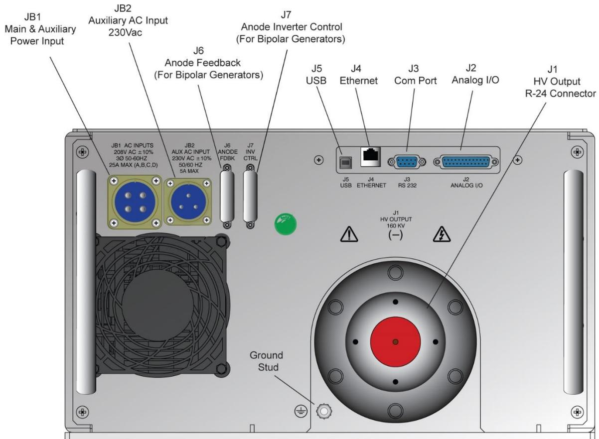
XR V160 (6kW) Rear Panel Connections
