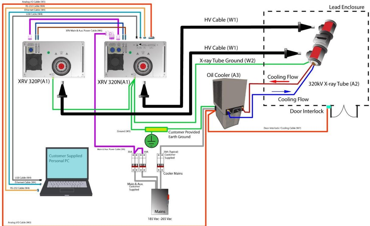
Typical Bipolar System (Minimal Requirements)
