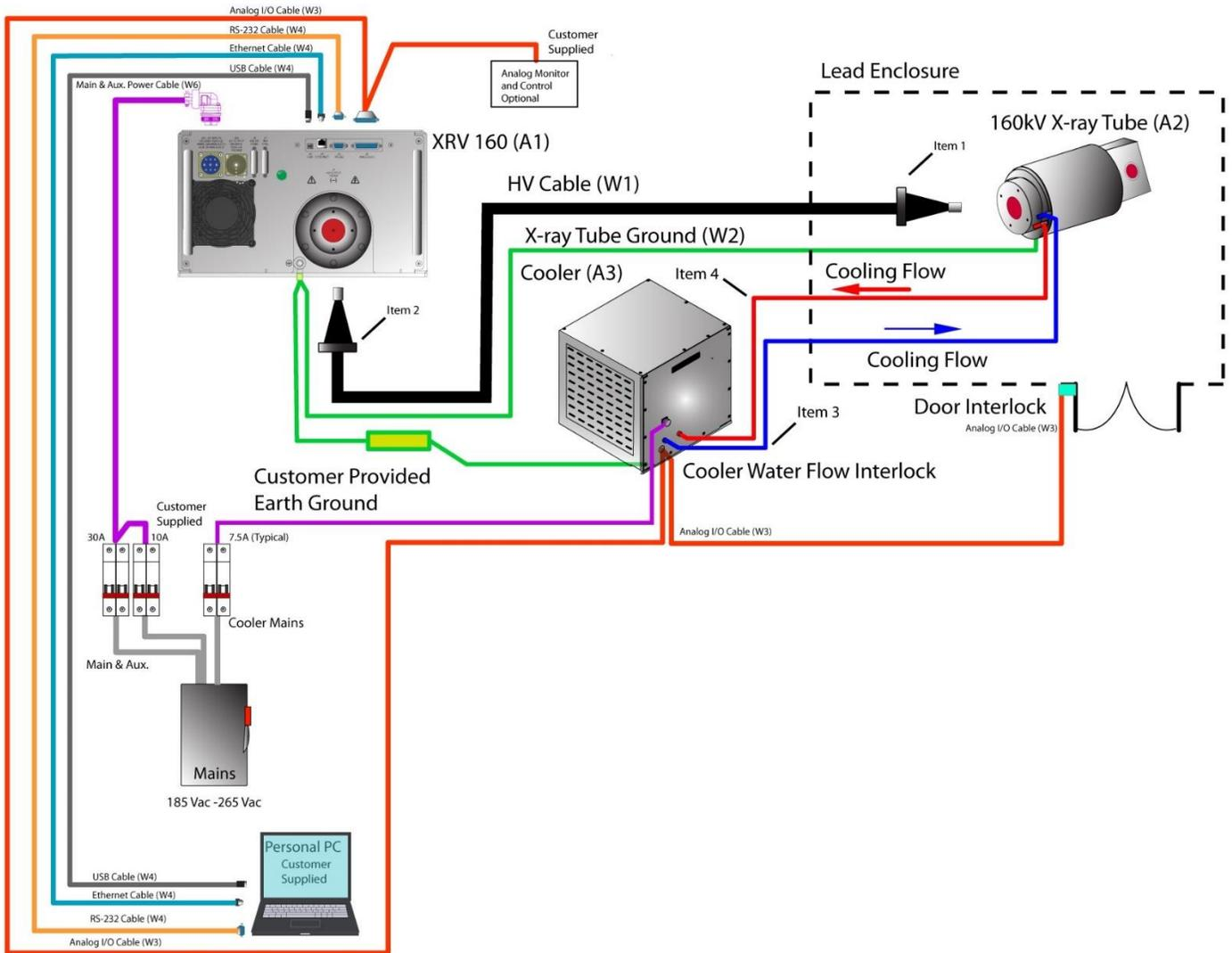
Typical Unipolar System (Minimal Requirements)
