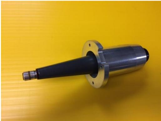
R28 test plug useful for evaluating or troubleshooting XRV225 model generators or X-ray tube functionality. The plug is inserted into the high voltage receptical and allows for operation of the XRV Generator without the X-ray tube load.
