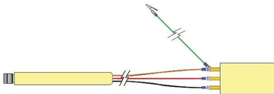
XRV X-ray tube filament calibration tool utilizing a unique adapter between the high voltage cable plug and the XRV Generator for X-ray tube filament current calibration and verification. For use with both the XRV160 and XRV225 models. Customer supplied ampere meter is required.
