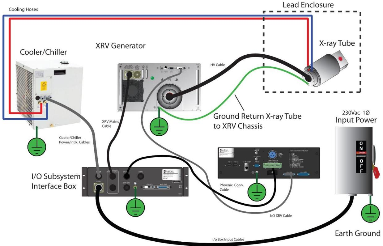
XRVC Controller, I/O System Interface Box, Cooler/Chiller, XRVC Generator and X-Ray Tube Setup for 4kW System
