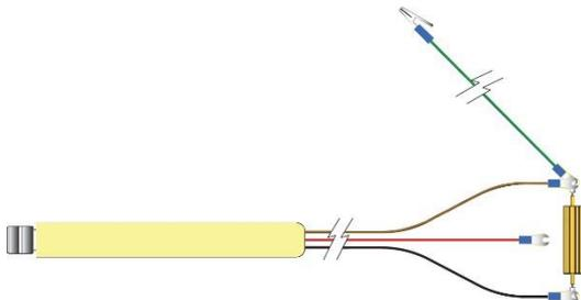
XRV filament power supply calibration tool utilizing a resistive load for filament current calibration and verification. For use with both the XRV160 and XRV225 models. Customer supplied voltmeter is required.
