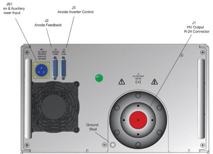
XR320 and XR350 Anode Rear Panel Connections
