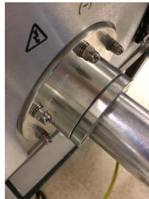
Insert HV plug in XRV & tighten flange screws
