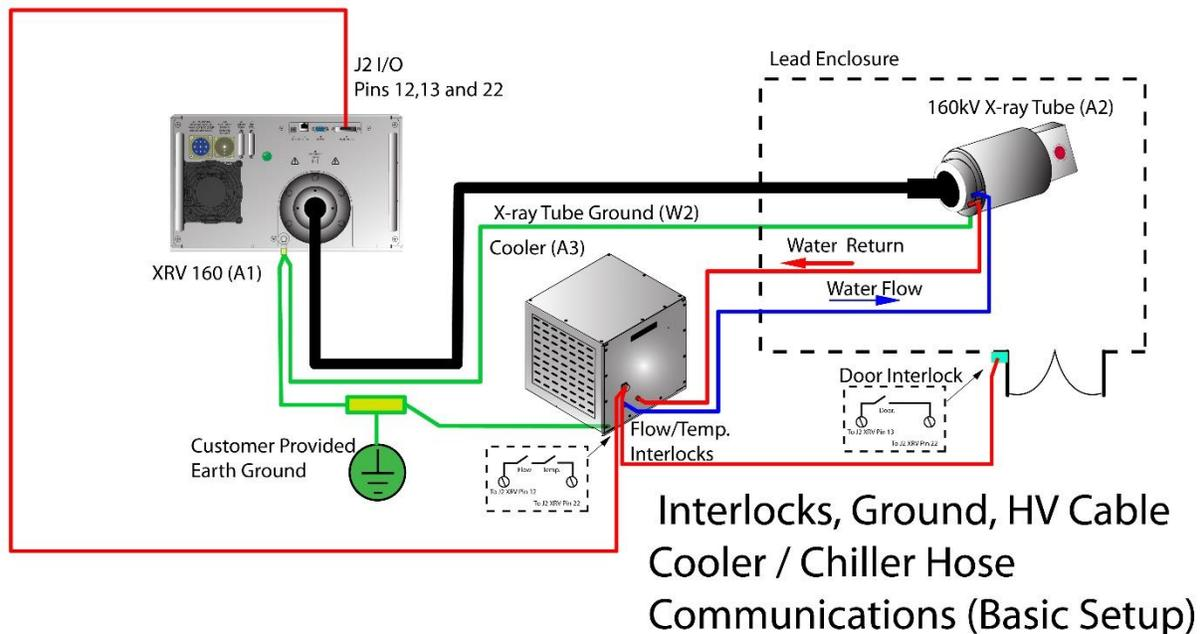
The next step is to choose the type of communication used for the control of the XRV Generator. There are three communication interface options including a Com Port RS-232, Ethernet Connection, and USB connection. The most commonly used is the RS-232 Com Port Connection. The connection consists of a customer supplied cable and the XRV Generator communication software selection.
