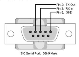
Figure 1 – J3, RS-232 DB-9M pinout (front view)
