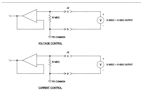
Figure 3.2 Local Programming via External Voltage Source
