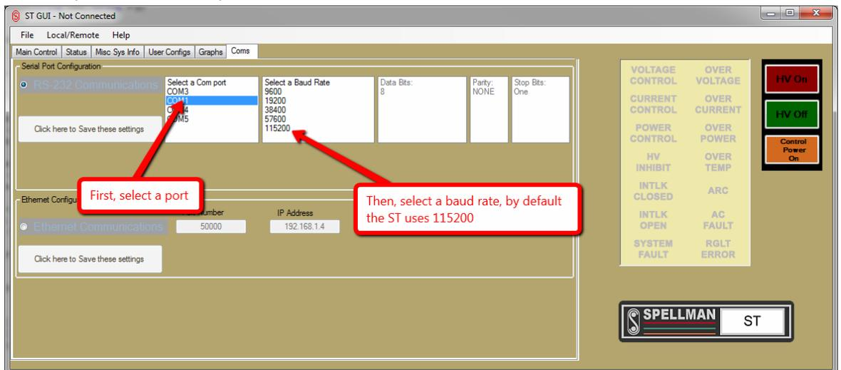
5. Select the baud rate in the same manner by clicking on it with the mouse, note that the default baud rate for ST units is 115200, and this is the option you should select unless you have specifically requested a different baud rate. Once selected, you will be presented with an option for selecting the Data Bit number.
