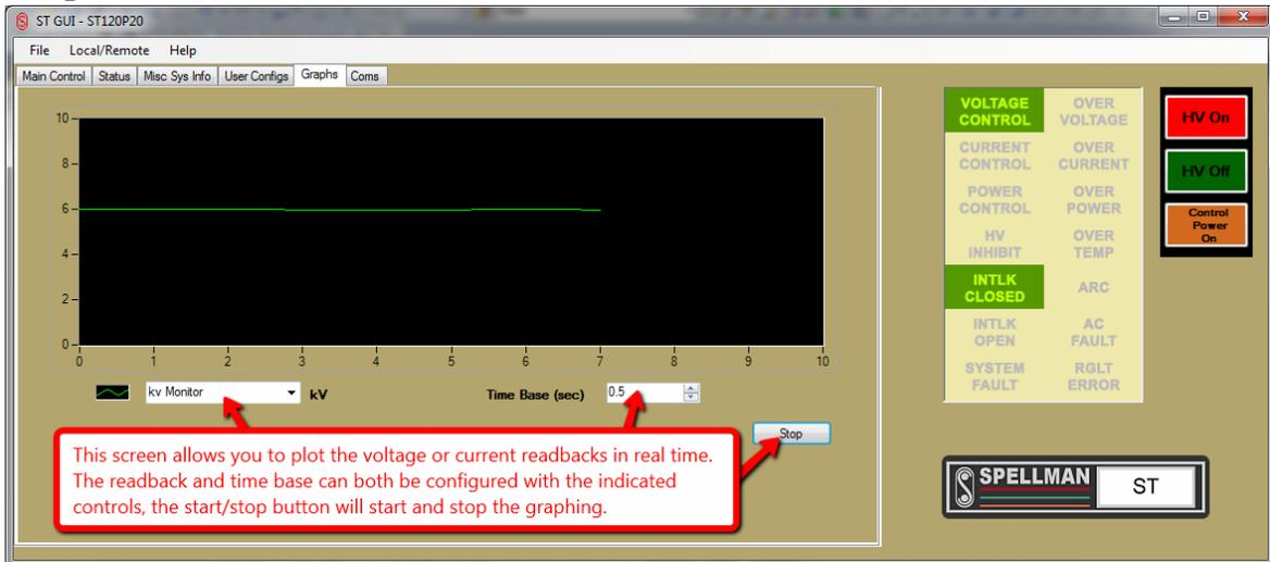
This tab allows real time graphing of the KV, mA or temperature read back. A selector is available to choose which of the three to display, and another selector allows the update rate to be specified in seconds. A start/stop button will start and stop the graphing.
