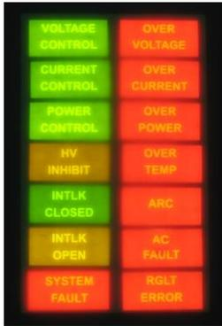
**VOLTAGE CONTROL:** Indicates the output voltage regulator circuit is maintaining voltage regulation.
