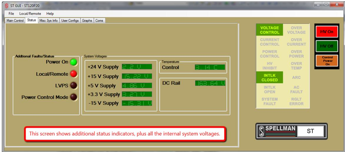
This tab shows a variety of status indicators including the state of the control power, local/remote mode indicators, the Low Voltage Power Supply problem indicator and a variety of housekeeping voltages in the Low Voltage Power Supply.
