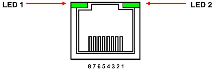
Figure 2 – JB9, Ethernet RJ45 Jack (front view)
