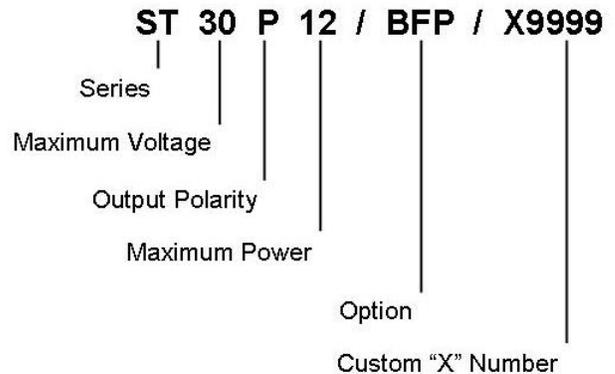
The model number of the power supply describes its capabilities. After the series name "ST" is:
