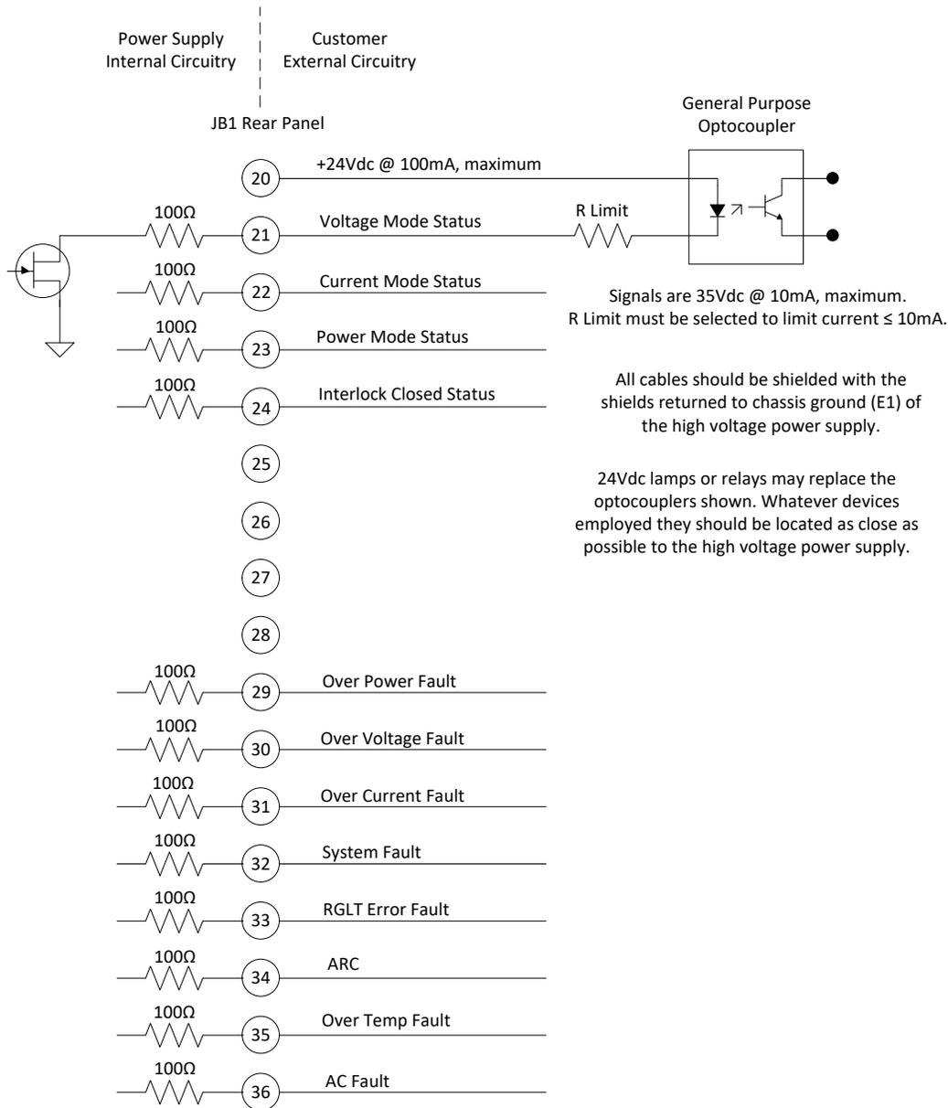
**Figure 3.9 Remote Status and Fault Indicator Interface**
