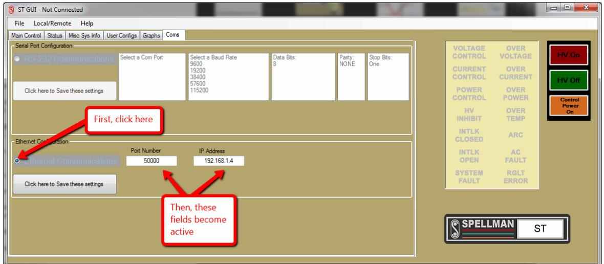
4. The default address and port number are automatically entered for you in the field, if you requested a different configuration with the unit, or have changed the units settings in the past, enter the correct information here. If you did not request a different configuration and you are unable to use the default settings, please contact Spellman High Voltage to address the situation.
