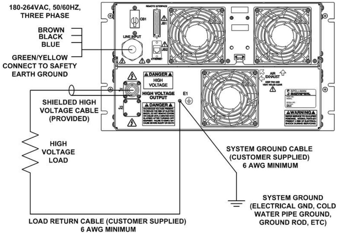
**Note: 400VAC units do not have an internal circuit breaker. The service connection to these units must be protected by an appropriately rated and circuit breaker protected power connection.**
