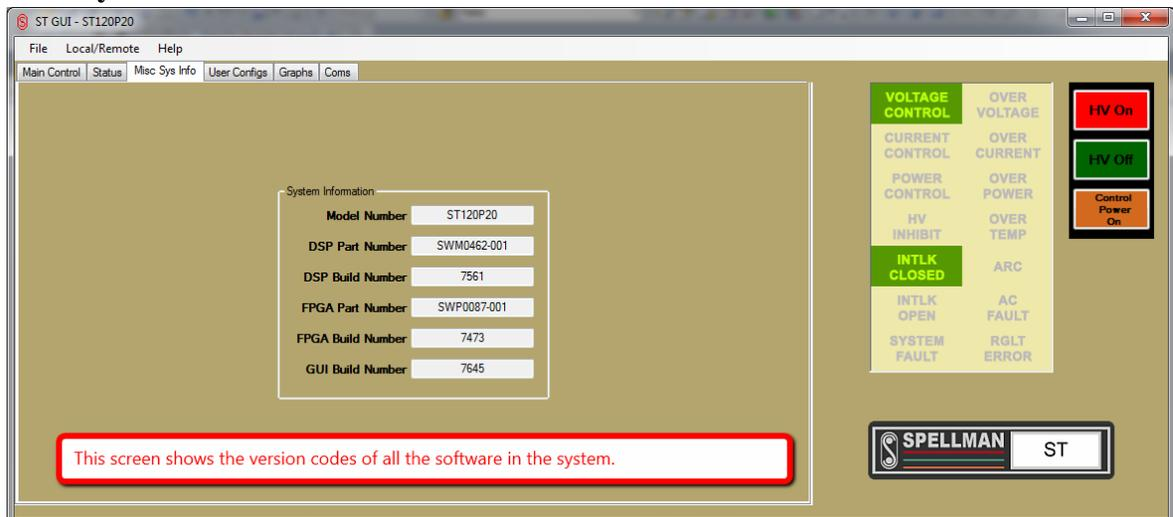
This tab indicates the model number and software version information for the power supply, as well as the desktop GUI version currently running.
