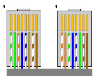
Figure 4 – Crossover Cable for Direct Connection
