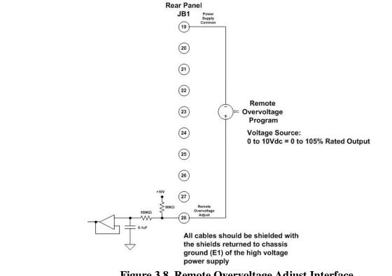
Figure 3.8 Remote Overvoltage Adjust Interface
