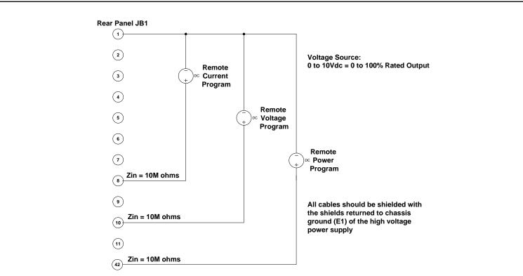
Figure 3.2A Wiring Diagram for Remote Programming via Voltage Source
