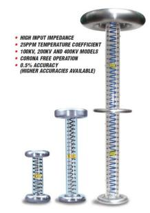
High voltage dividers for precise measurements of output voltage with accuracy up to 0.1% are available from Spellman. The HVD-100 is used for voltages up to 100kV, the HVD-200 measures up to 200kV and the HVD-400 measures up to 400kV. The Spellman HVD divider is designed for use with differential voltmeters or high impedance digital voltmeters. The data sheet for Spellman's series of HVD dividers can be viewed by clicking here.
