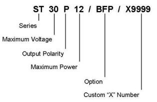
The model number of the power supply describes its capabilities. After the series name "**ST**" is:
