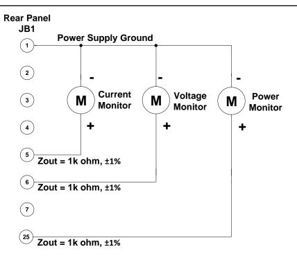
**Figure 3.3 Remote Monitor Test Point Designations**
