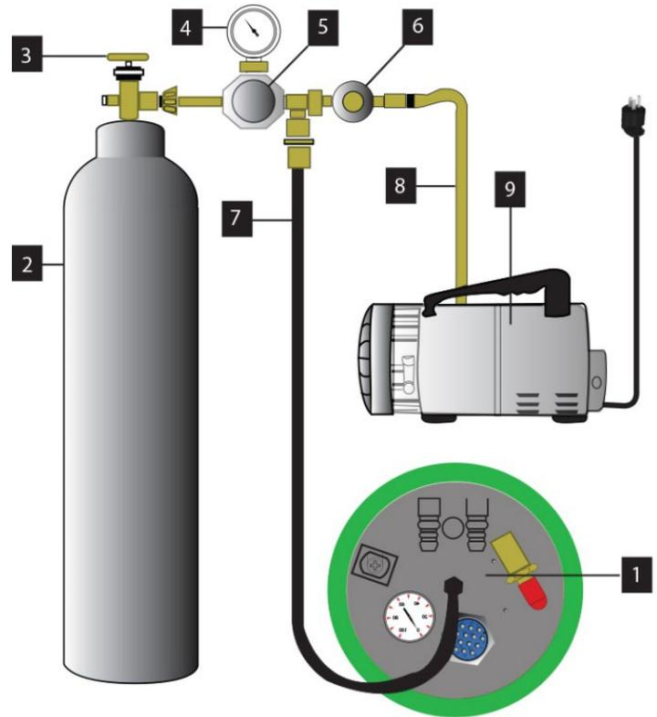
Figure 7-1 Tube Head Pressurization Setup
