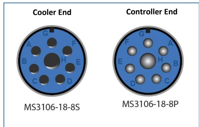
Figure 4-12 Interlock (Controller)
