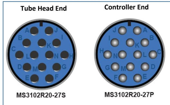
Figure: 4-8 Tube Head Power Cable
