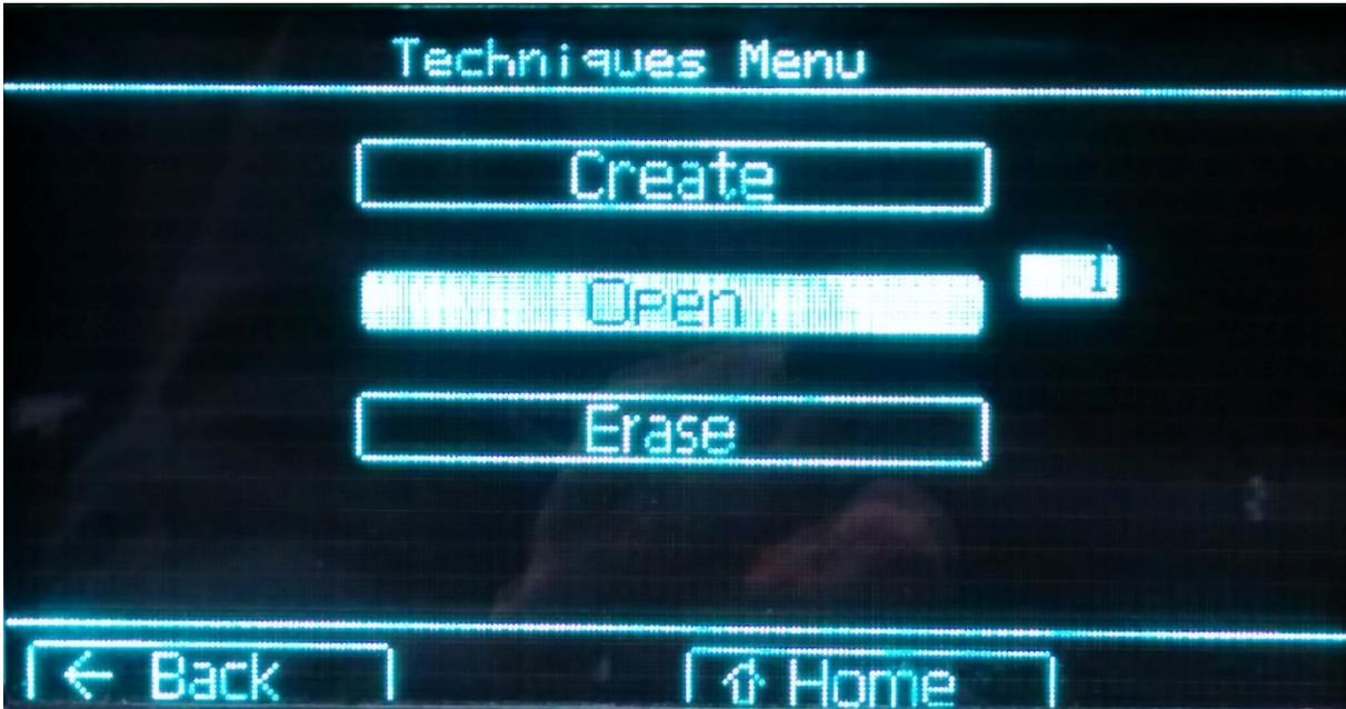
If no valid technique exists for the number selected, the error message “No valid data for technique #” will appear. Valid values for the number field are from 1 to 200.
