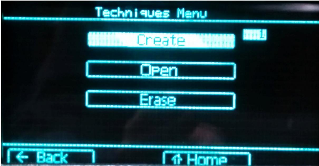
If a technique is to be opened, a number field will appear which must be set. This will select the technique to open. Only valid technique numbers can be selected.
