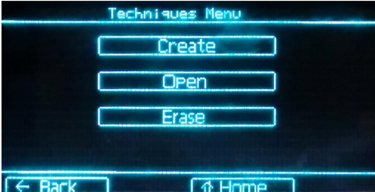
If a technique is to be created, a number field will appear which must be selected. This will be the number assigned to the new technique. If a technique with the number already exists, it will be overwritten. Valid values for the number field are from 1 to 200.
