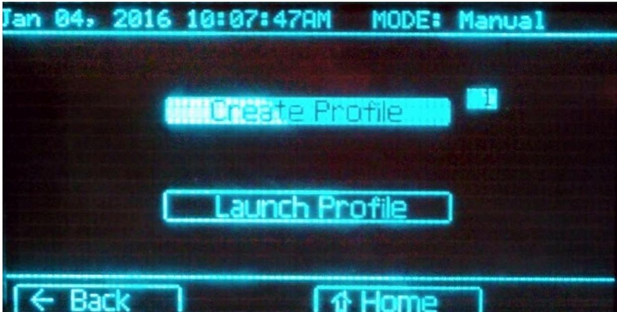
Seasoning “Auto-Warming” is important to preserve the x-ray tube. It is required whenever the tube is operated above 80 kV and four hours have elapsed since the x-ray tube was operated at the level required for the next exposure, or when operating a new tube having less than ten hours of operation. Tubes having been previously operated, but not run over 80 kV for 30 days or longer, must be treated as new tubes.
