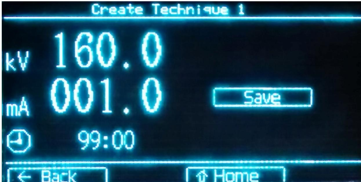
When the technique is saved, an acknowledgement message of "Technique # data saved!" will be displayed.
