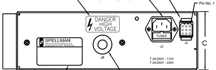
Identification Label High Voltage Output AMP: LGH4I Conn. or Flying Lead 24" (Customer Specified)
