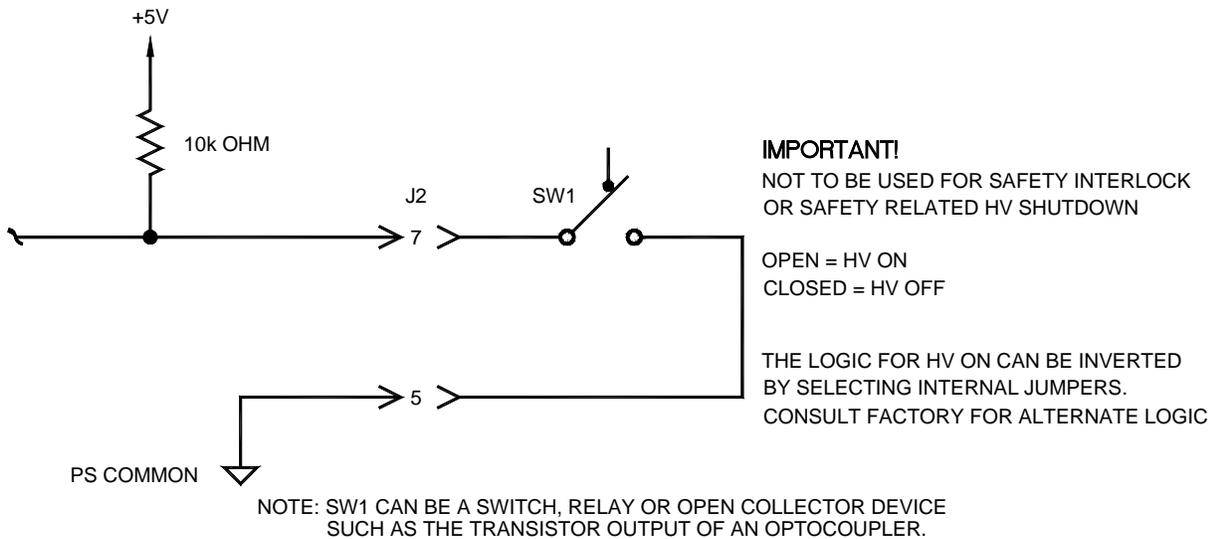
**Figure 3.4 HV ON/OFF Control**
