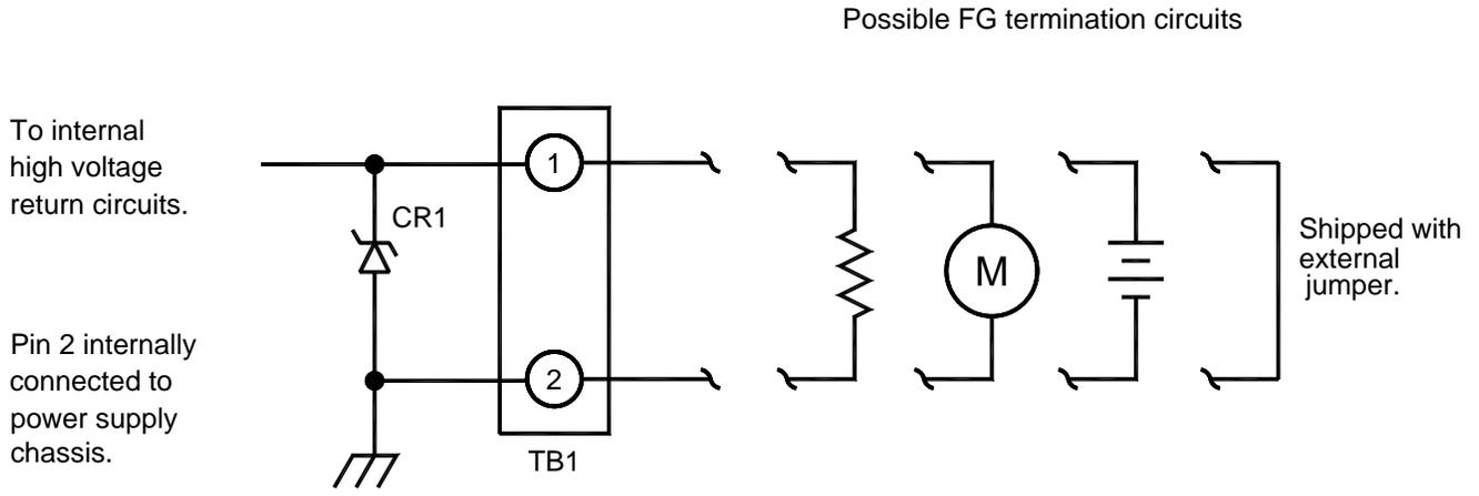
CR1- Polarity dependent on output voltage polarity. Zener voltage is 15V standard. Up to 50V is available. Consult factory.
