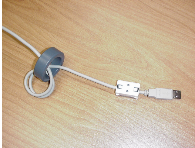
Figure 7 - Example of a USB Cable Using Ferrites
