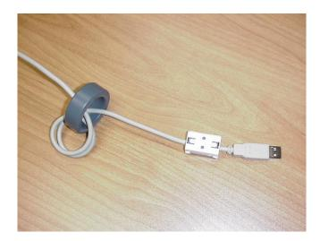
Figure 8 - Example of a USB Cable Using Ferrites
