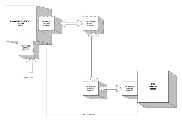
**Figure 7 – Block Diagram of USB Cable Utilizing Ferrites** Ferrite beads should be attached to the USB cable next to the connectors – both sides should be installed. In extreme cases ferrite cores may be added where the cable is looped 3 or 4 times around the core as shown in figure 8. Cores of 1.5 to 2 inches should be used at both ends of the cable.
