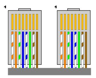
Figure 5 – Standard Straight Through Cable – Standard CAT5 Patch
