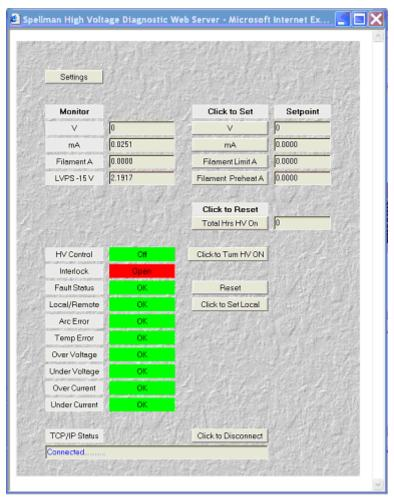
Figure 11 - Control and Monitor Applet
