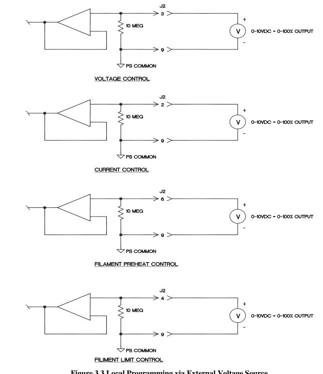
Figure 3.3 Local Programming via External Voltage Source
