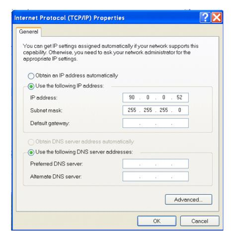
Figure 20 - TCP/IP Properties
