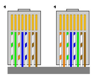
Figure 4 – Crossover Cable for Direct Connection
