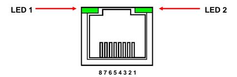
Figure 2 – J5, Ethernet RJ45 Jack (front view)
