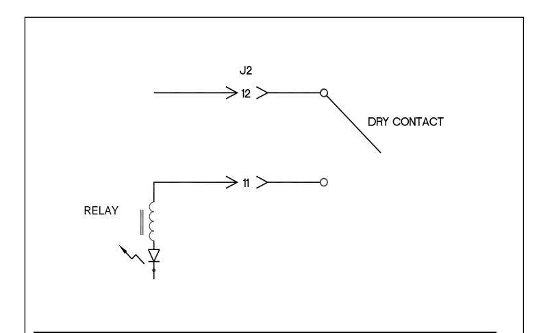
Figure 3.5 Enable/Interlock Logic Control
