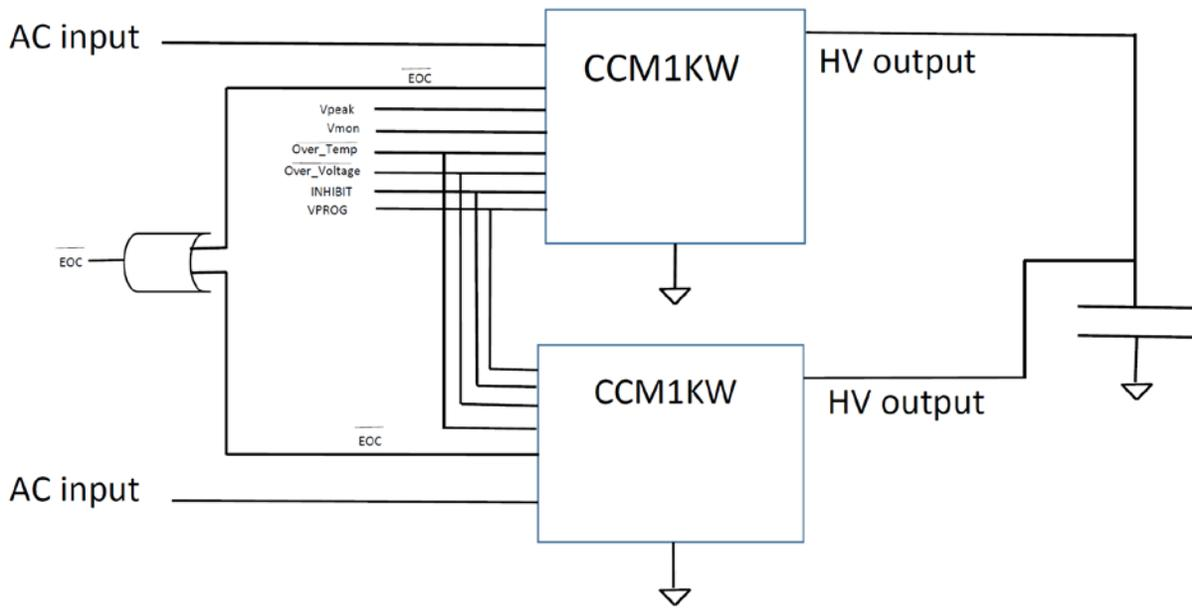
Figure 3.2 Parallel Operation
