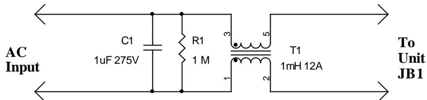
Figure 6.1 Class B Conducted Emission Input Filter Circuit.
