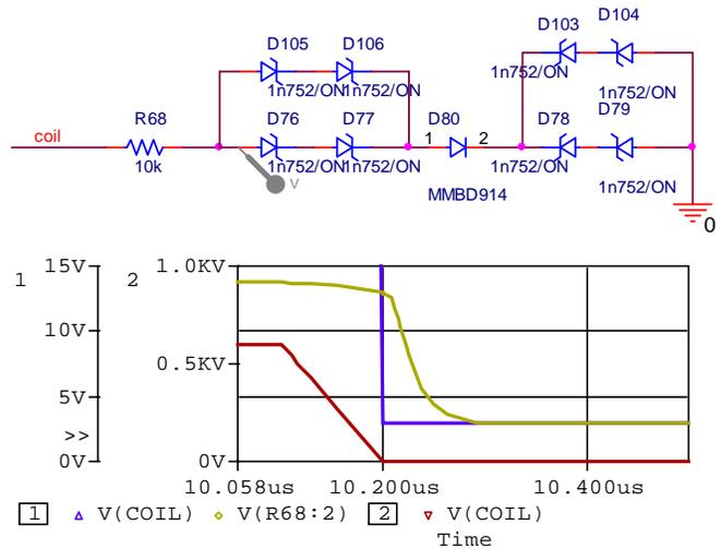
Fig. 4. Blocking Zener diode capacitance using a fast diode. Circuit excited by source V1 Fig. 2.
