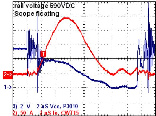
Fig. 3. Measurement of collector-emitter voltage  $V_{ce}$  of CM300DC-24NFM Powerex IGBT using circuit Fig. 2. TDS 3024B scope is floating. In this and further plots, waveform notes carry scale information and types of probes used.
