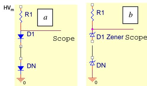
Fig. 1. Schematics of basic nonlinear voltage dividers.
