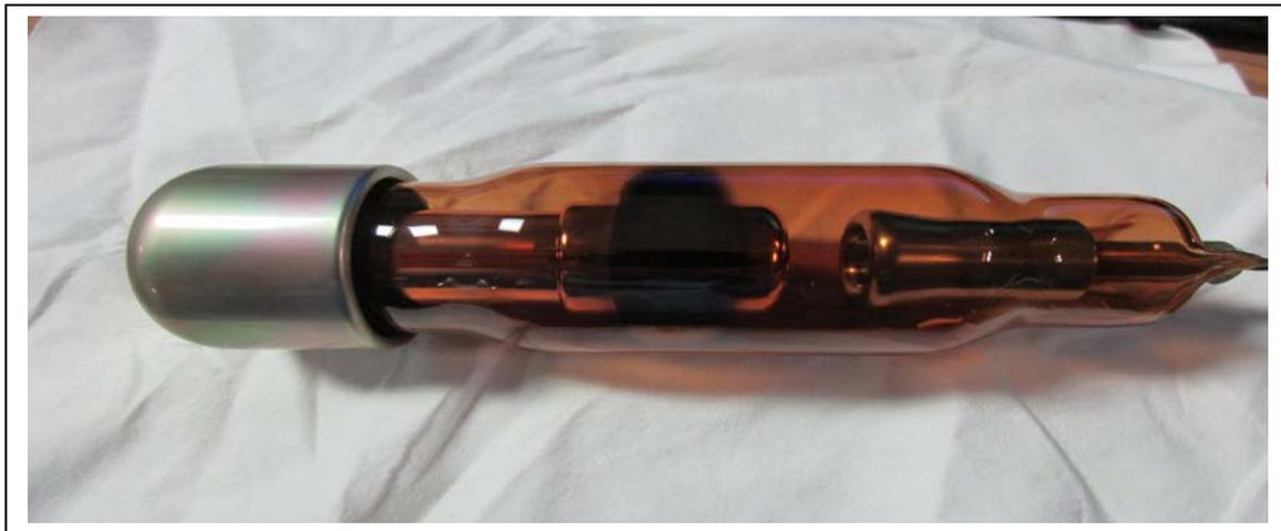
**Figure 9:** An X-ray tube operated in a hot oil environment with a thin layer of carbonized oil etched onto its surface.
