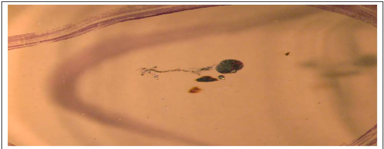
**Figure 2:** Magnified arcing area on the glass, showing a damaged tube wall.
