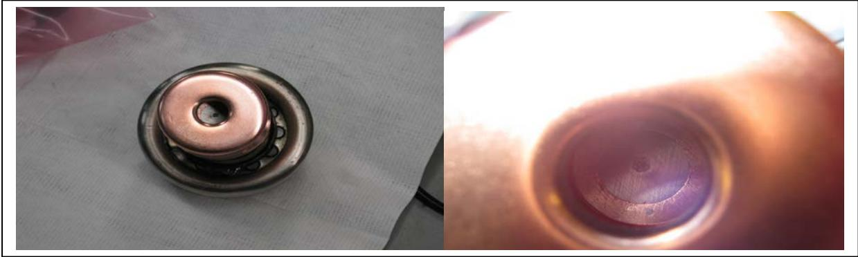
**Figures 10, 11:** Focal spot damage caused by inadequate anode cooling and thermo-mechanical stress
