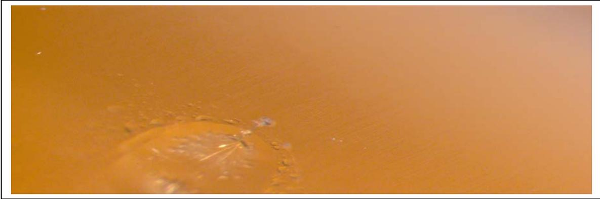
**Figure 6:** Tube glass puncture caused by high electrical stress.
