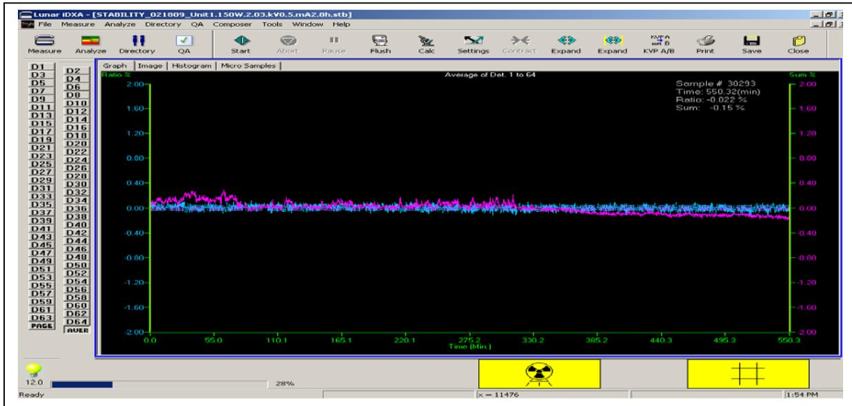
**Figure 13:** Performance of a compensated X-ray source. The traces show the sum of low and high energy photons (purple trace - proportional to the equivalent mA stability) and ratio of high and low energy photons (blue trace – proportional to the equivalent kV stability).
