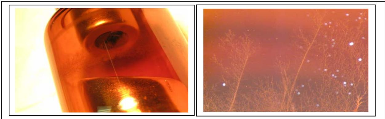
**Figures 7, 8:** Glass envelope etched in the presence of high E-field.
