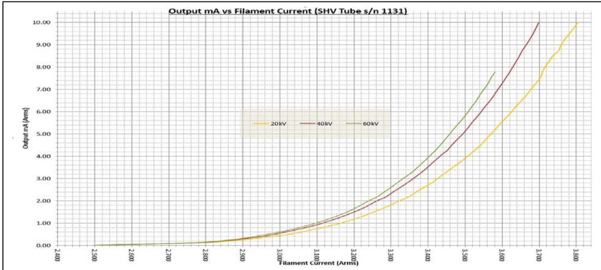
**Figure 3:** Typical X-ray tube characteristics. When the tube voltage decreases, in order to maintain constant output current, the filament current must increase.
