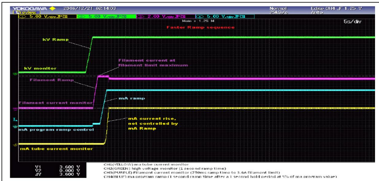
**Figure 4:** Filament and output currents during fast ramp.
