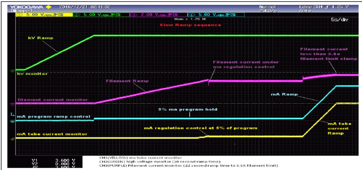
**Figure 5:** Optimized Filament Current Ramp Up Reduces Stress on the X-ray tube Filament.
