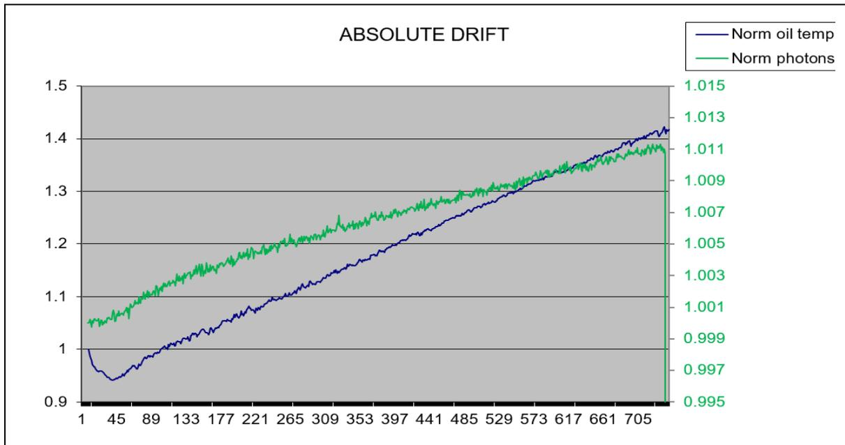
**Figure 12:** X-ray dose drift as a function of operating temperature. Horizontal axis shows time in seconds.
