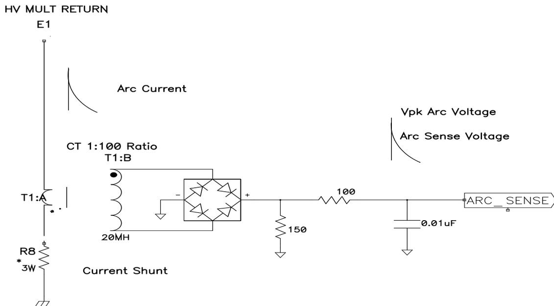
**Figure 2a:** Example of an Arc Sensing Circuit in an X-Ray Generator
