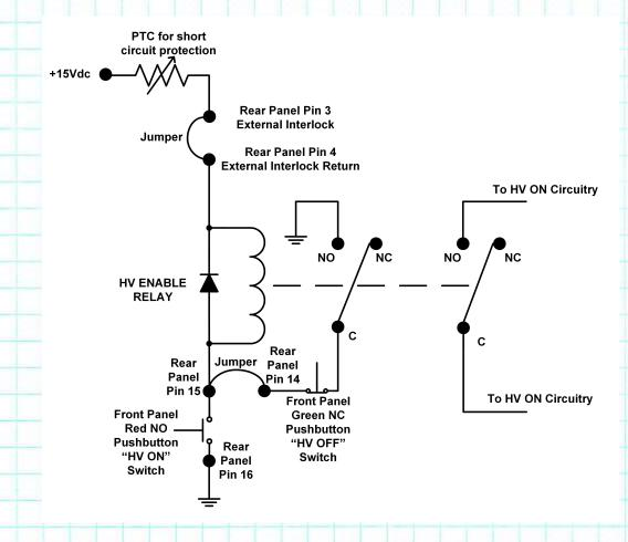
The above diagram shows a simplified SL HV ON/OFF schematic, functionally it is correct but it does not show all the actual circuitry. In reality, there are additional interlocks and circuitry that can turn off the high voltage if a fault is detected. The switches shown are the front panel HV OFF and HV ON switches. The three points on the simplified schematic are brought to the rear panel and are identified as pin 14, pin 15 and pin 16:
