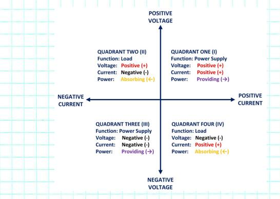
Output current and voltage are shown on the respective horizontal and vertical axis and four operational quadrants are created.
