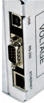
Closeup showing digital interface connectors
