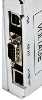
Closeup showing digital interface connectors
