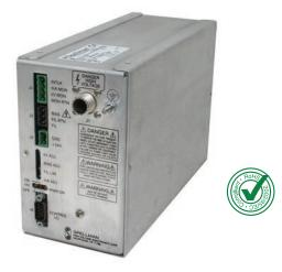
Spellman's XRM Series of regulated X-ray power supplies offer output voltages to 65kV and incorporate a filament supply which provides regulated dc current adjustable between 0.3A and 3.5A at 5.5V. High voltage and filament current can be linearly ramped up. The XRM incorporates local and remote programming, monitoring, safety interlock, short-circuit and overload protection.
