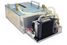
Spellman's XRB80PN320 Monoblock<sup>®</sup> X-Ray source is designed for OEM applications powering its internal X-Ray tube up to 80kV at 320W. Features like small package size and RS-232 digital interface simplify integrating this Monoblock<sup>®</sup> into your X-Ray system. Standard models are available with fan shaped beam geometry. Proprietary emission control circuitry provides excellent regulation of X-Ray tube current, along with outstanding stability performance.
