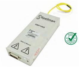
The XMPF is a modular 10kV @ 5W X-Ray generator designed to drive a floating filament X-Ray tube via closed loop filamentary control of the 0 to 500uA emission current. The floating filament supply is rated at 0 to 0.42 amps @ 3.5Vac. The filament supply features an adjustable 0 to 0.42 amp filament limit.
