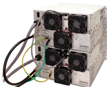
Rear panel showing connections for parallel operation
