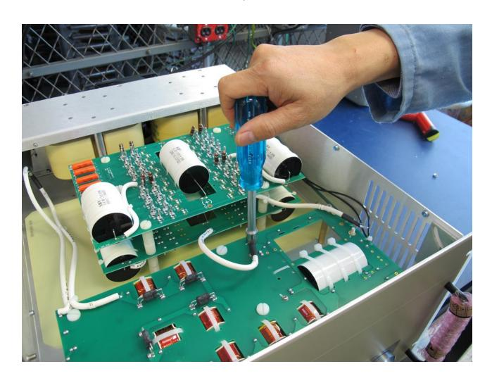
Loosen/remove wire #2 nut and lug.
