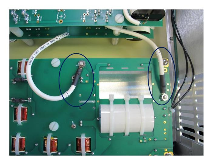
Uncrossed Wires = POSITIVE OUTPUT POLARITY
