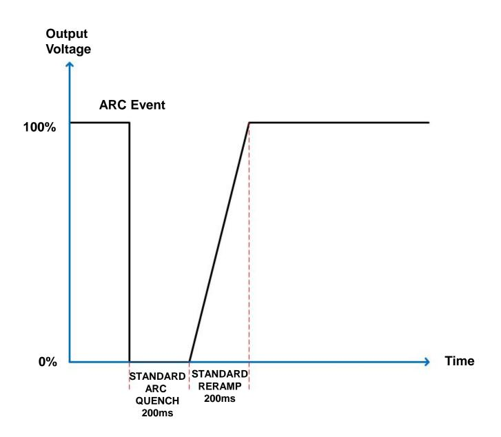
If 4 arcs occurs in a 10 second time period the power supply will trip off with an "ARC" fault latched on the front panel diagnostic display. User intervention is required to clear the fault and reapply high voltage. If 4 arcs do **not** occur in the 10 second time period, any counts loaded into the counter are cleared. A new 10 second time window is opened when the next arc occurs and the cycle repeats.
