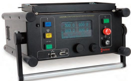
The SPX microprocessor-driven control unit provides automatic warm-up and comprehensive self-diagnostic circuitry. Memory to store and recall exposure techniques is standard and the last set of exposure parameters is retained before powering down. The SPX is adjustable in 1kV and 0.1mA increments. Exposure duration can be set from 1 second to 99 min 59 seconds in 1 second increments. There are three models to choose from: 160kV, 200kV and 300kV.
