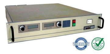
Spellman's SL2KW Series of 2kW high voltage power supplies are designed to meet uncompromising performance standards in a minimum of space. Their circuitry includes a resonant high frequency inverter with proprietary control which provides fault-free operation in extreme transient and arcing environments with greater than 85% efficiency. These full featured supplies are available in a wide range of outputs with many options.
