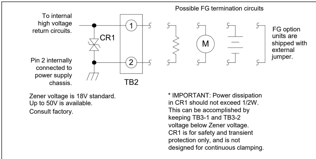
**FGLL Floating Ground Low Leakage**
