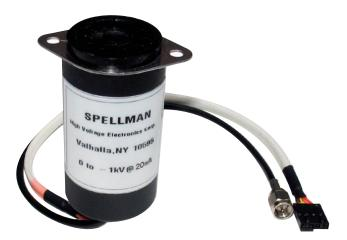
Spellman's PMTS is a custom designed high voltage power supply and integrated mounting socket for standard 1.125 inch (28mm) side-on photomultiplier tubes. Ten equally divided, incremental output voltages are generated and provided via the use of a 10 stage voltage multiplier arrangement.
