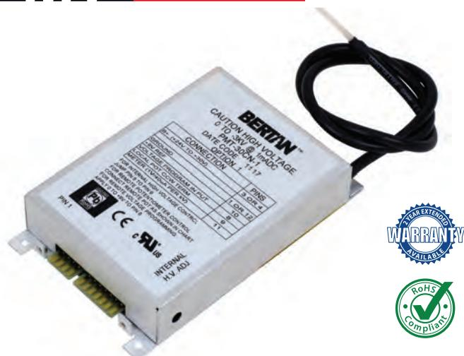
Spellman's Bertan brand of PMT modular high voltage power supplies offer well regulated, fixed polarity outputs up to 7.5kV, which operate off a low voltage DC input voltage. These fully enclosed modules are specifically designed with proprietary linear power conversion techniques to provide exceptionally low ripple and noise. The PMT is ideal for precision applications including: photomultiplier tubes, solid state detectors and ultrasonic transducers.
