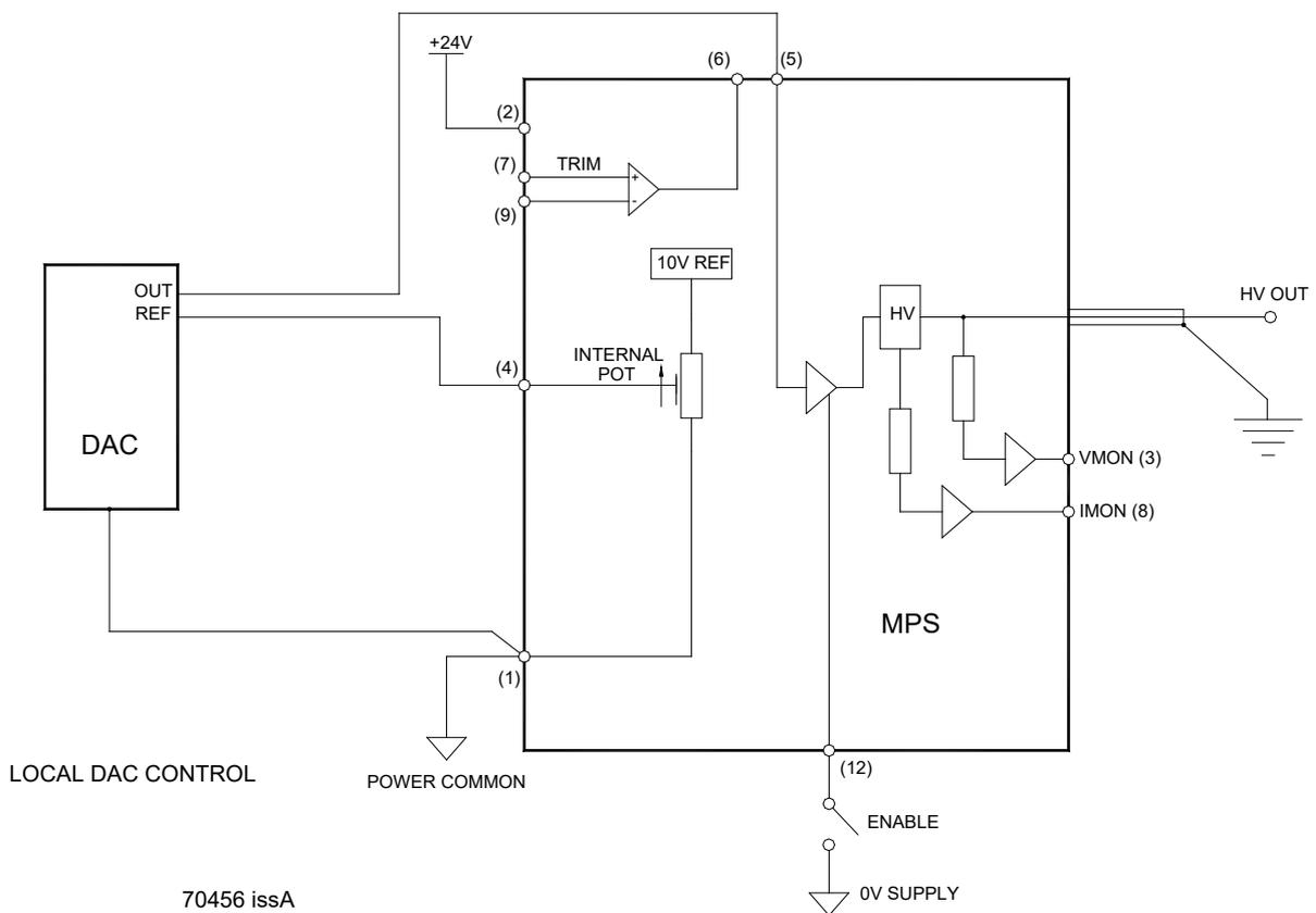
Q11. How do I connect the unit for Internal potentiometer control?
