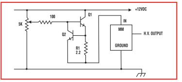
Circuit 2 This circuit is designed for fixed output voltages below the normal output voltage and has a line regulation of 5%/V (typical) change depending on the zener.
