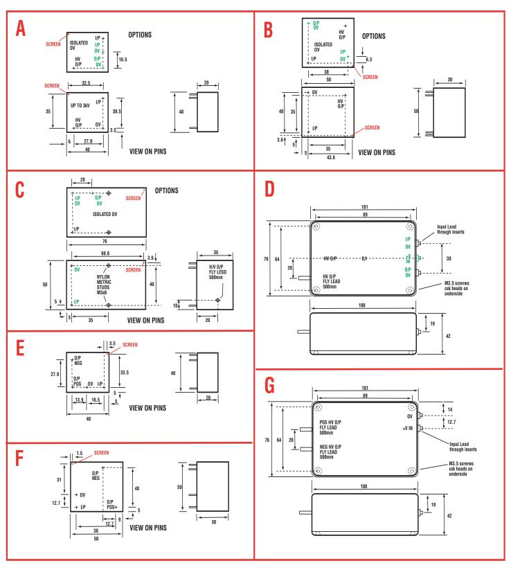
Standard configurations of housings for the MM Series modules. Refer to case size reference in specifications on page 1. Available options are shown in color; RED= Screen GREEN= Isolated I/P to O/P
