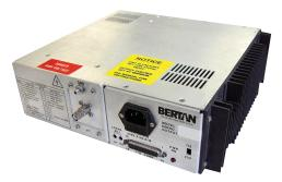
Spellman's Bertan brand of 825 Series high voltage power supplies provide well-regulated, fixed polarity outputs from 500 to 50kV that operate off a standard switch-selectable 115/230Vac input. The 825 Series is fully arc and short circuit protected. Excellent regulation specifications are featured along with outstanding stability performance.
