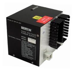
Spellman's Bertan brand of 606C modular high voltage power supplies offer well regulated, fix polarity outputs up to 30kV, which operate off a +28Vdc input (+24Vdc optional). These fully enclosed modules are designed for bench top or OEM applications like spectrometers, detectors, imaging and electron beam usage.
